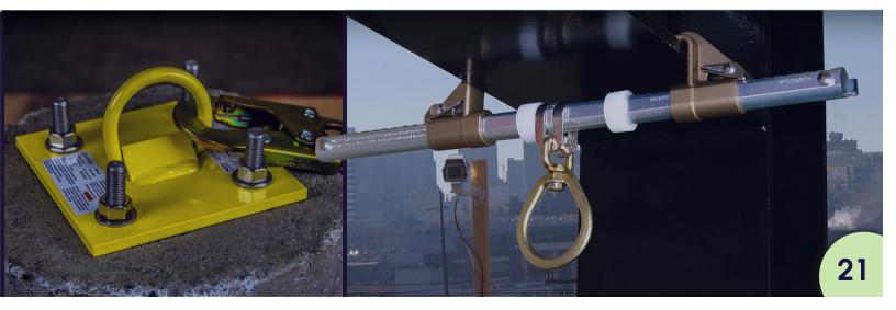
For static strength testing, both Type A and Type T anchors must withstand a minimum 5,000 lb. load. Type D anchors must withstand a static load between 2,700 lbs. and 5,000 lbs., and their deformation must be measured so that it may be accounted for in fall clearance calculations.
