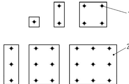
Fig. 4.23: Number of headed studs according to CEN/TS 1992-4-1 [1]
