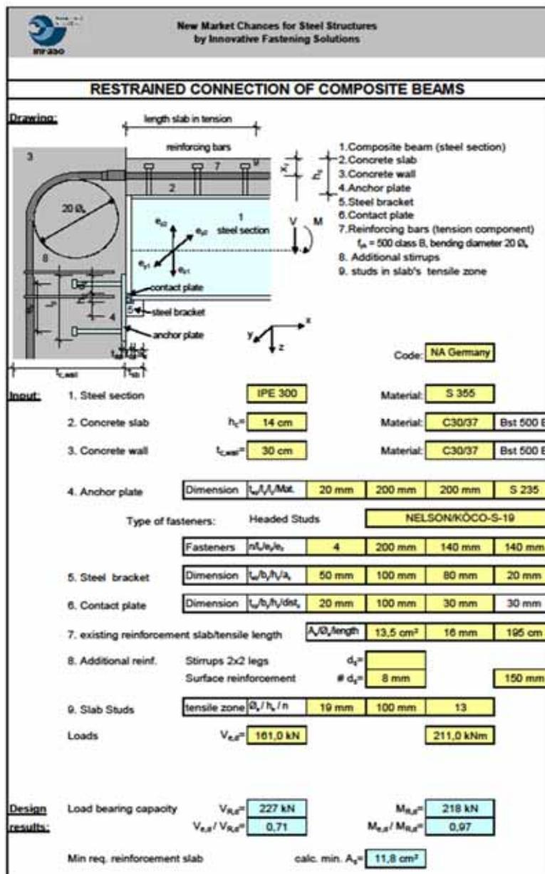
Fig. 3.9: Structural analysis of the restrained connection
