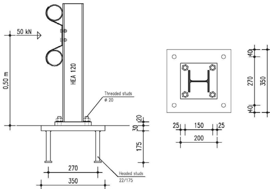
Fig. 3.10: Conventional joint solution of the safety fence
