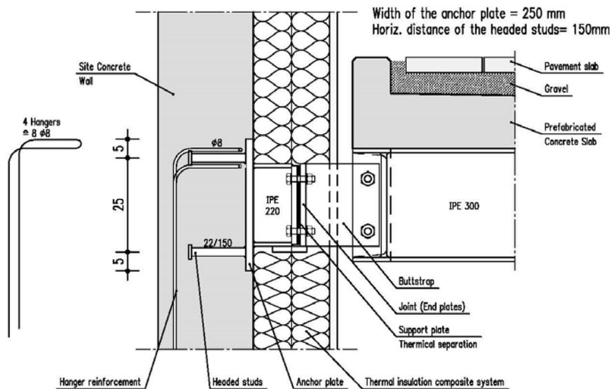
Fig. 3.19: Improved joint solution of the balcony construction
