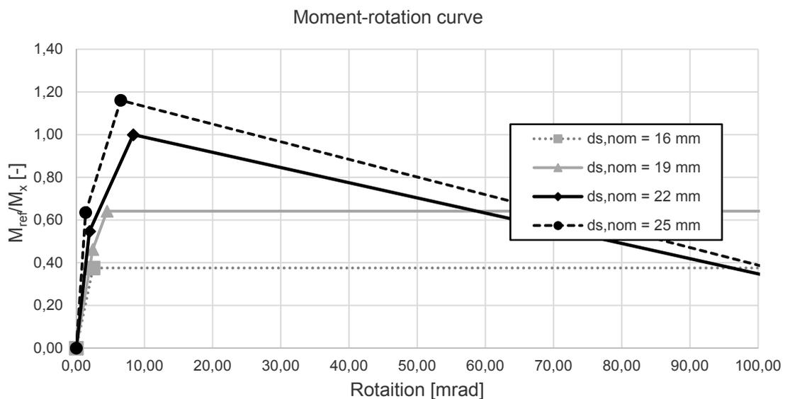
Fig. 4.17: Moment-rotation curve of the simple steel-to-concrete joint for variation of the diameter of the headed studs
