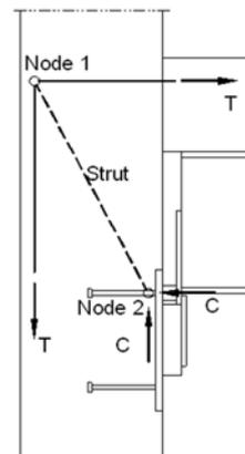
Fig. 2.7: Strut and tie model
