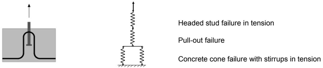
Fig. 2.9 Component headed studs with stirrups in tension
