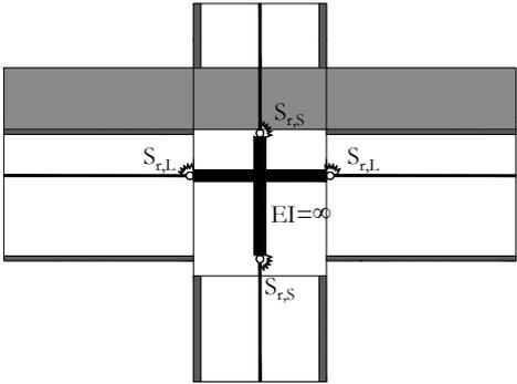
Fig. 7.1a Representation of joint by infinite rigid stubs
