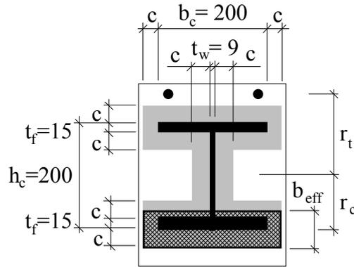
Fig. 9.23a The effective area under the base plate
