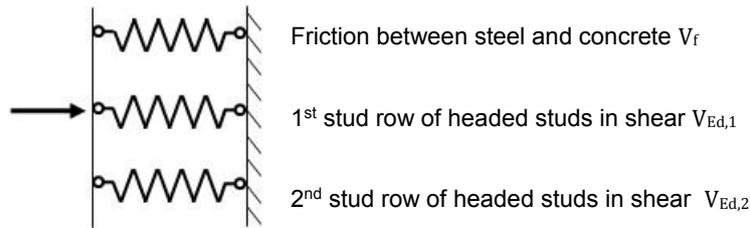
Fig. 5.7 Shear components
