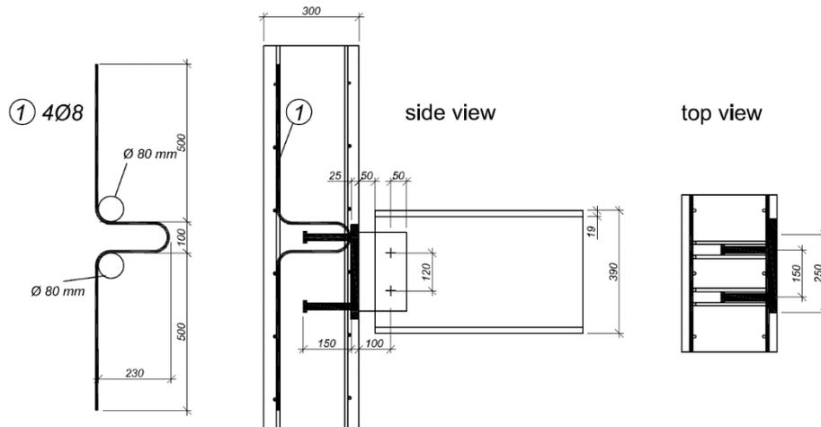
Fig. 9.27 Reinforcement
