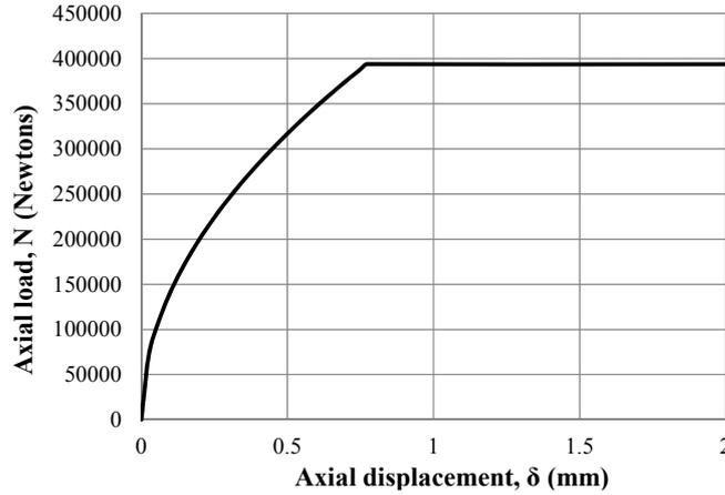
Fig. 9.10 Load-displacement behaviour of spring representing component RS
