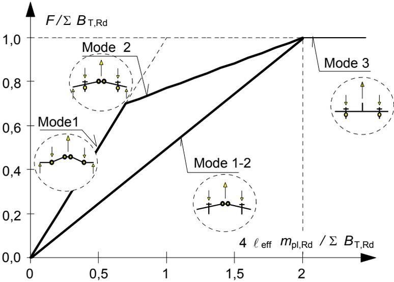
Fig. 4.8 Failure mode 1-2
