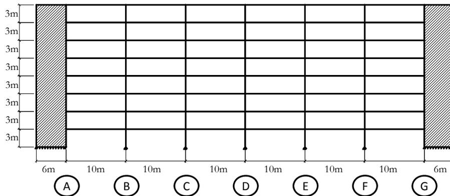
Fig. 7.6c Geometry of sub-structure III, car park building alignment 2
