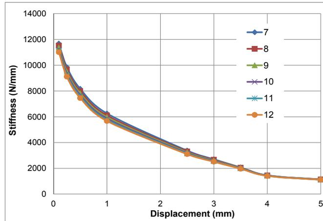
Fig. 4.7: Influence of pressing relation,  $m$  on stiffness of anchorage
