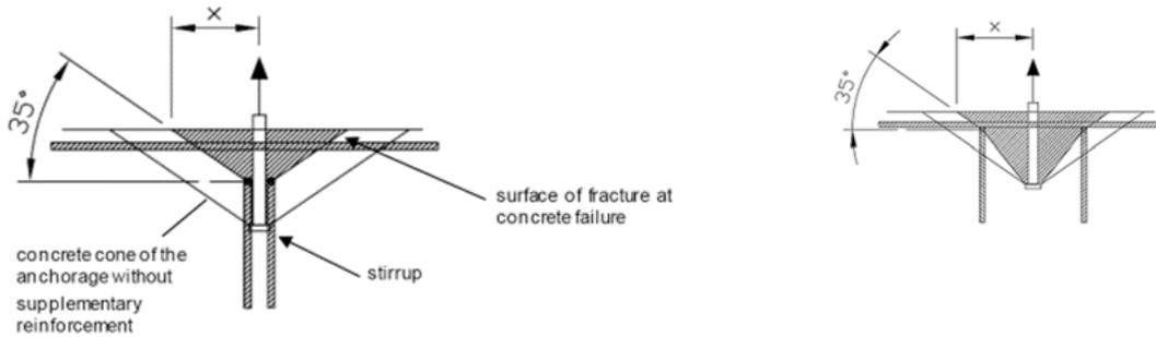
Fig. 3.4 Distance between the anchor and the crack on the concrete surface
