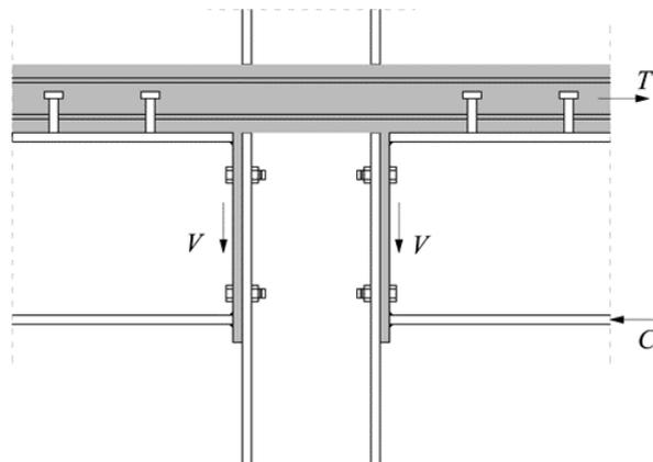
Fig. 2.8 Composite joint
