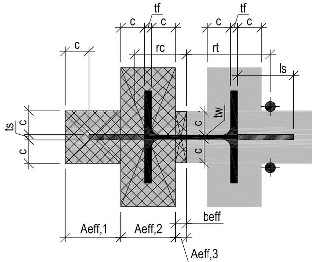
Fig. 9.18 The effective area under the base plate
