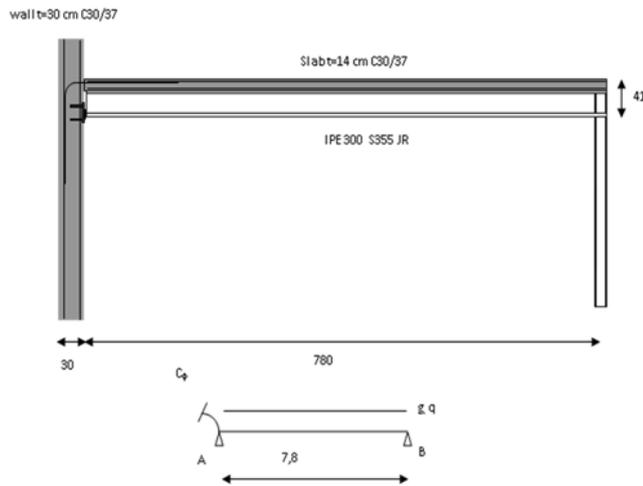
Fig. 3.1: Structural system
