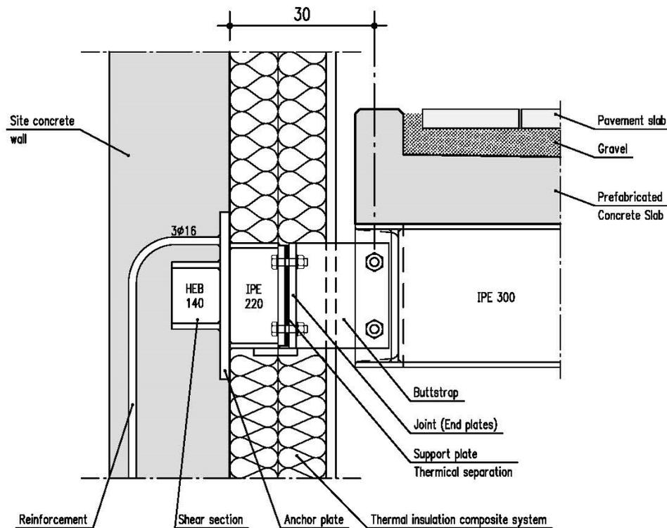
Fig. 3.18: Conventional joint solution of the balcony construction
