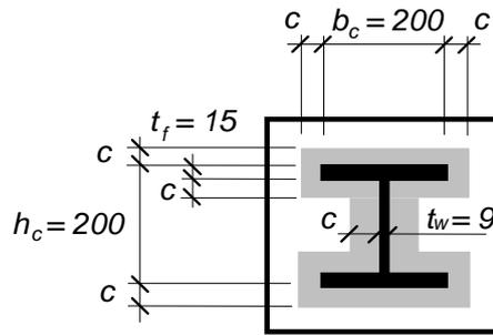
Fig. 9.2 Effective area under the base plate
