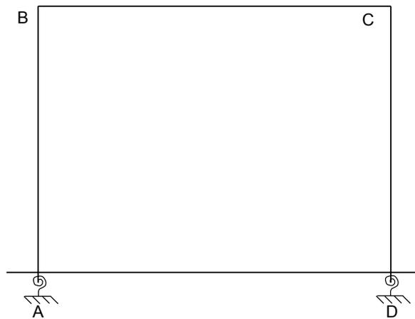
Fig. 9.44 Structural system with rotational springs
