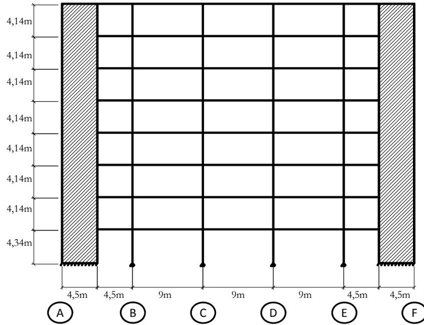
Fig. 7.6b Geometry of sub-structure II, Office building alignment 3
