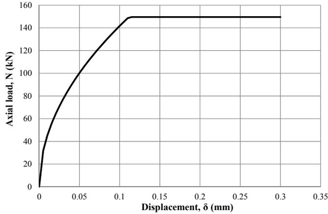
Fig. 9.11 Load-displacement relation of spring representing component RB
