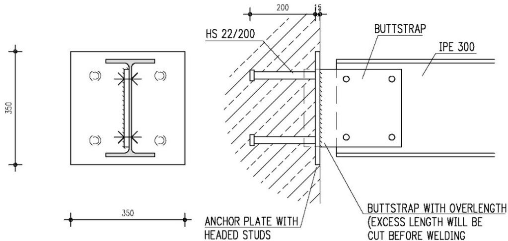
Fig. 8.4 Joint with possibility of adjustment
