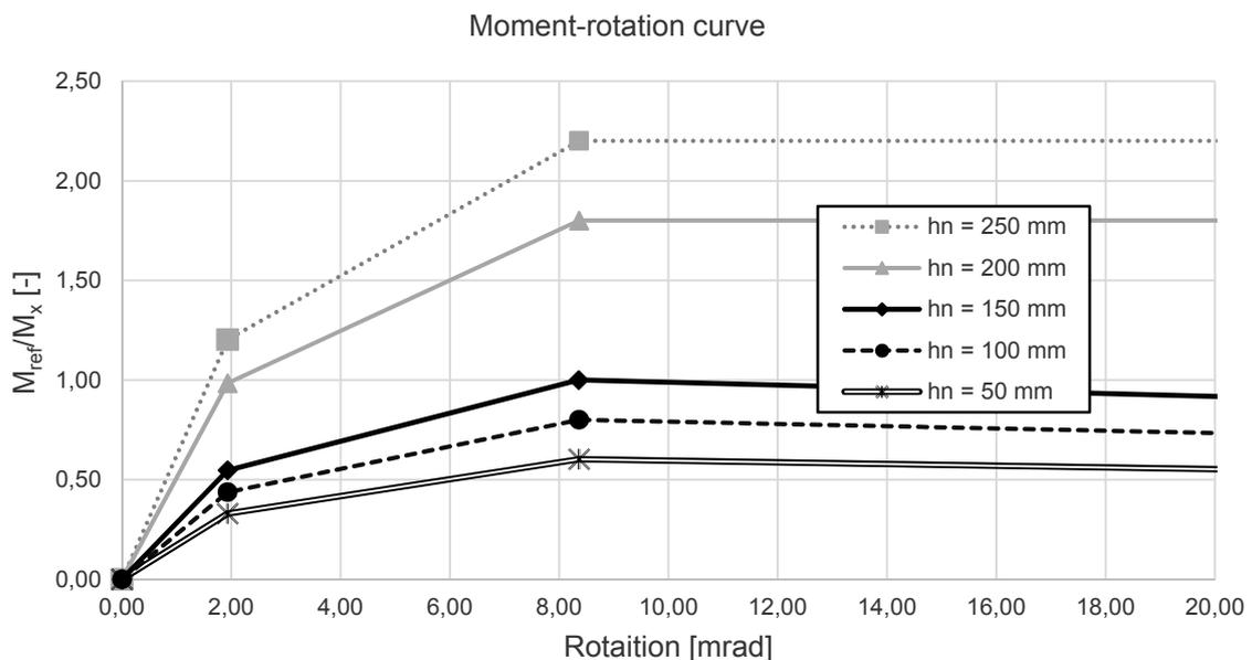
Fig. 4.18: Moment-rotation curve for variation of the eccentricity
