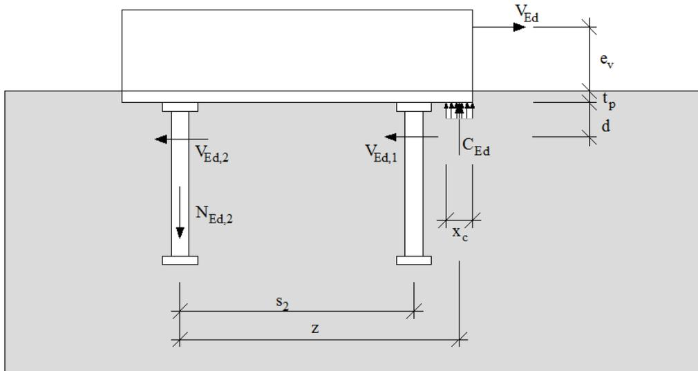
Fig. 5.5 Forces at the anchor plate caused by the shear force  $V_{Ed}$  and its eccentricity  $e_v$
