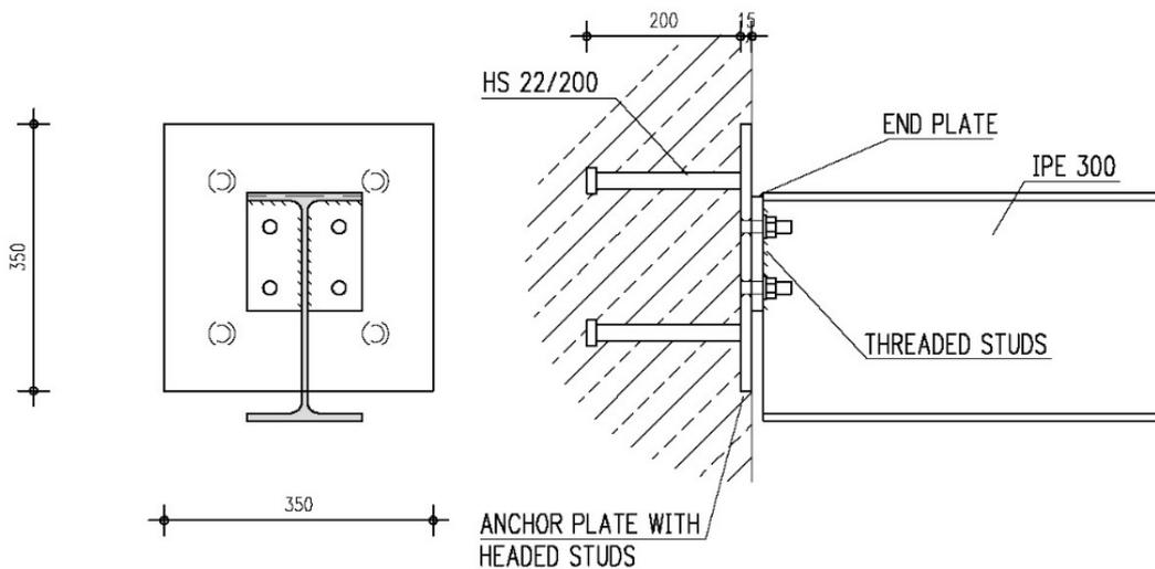
Fig. 8.5 Joint without possibility of adjustment
