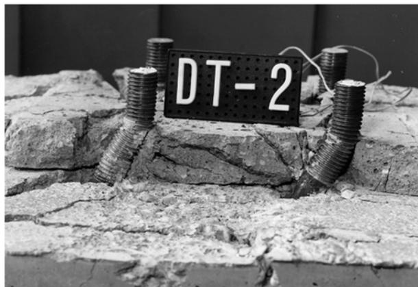
Fig. 4.20 Test specimen loaded by shear force and tensile force
