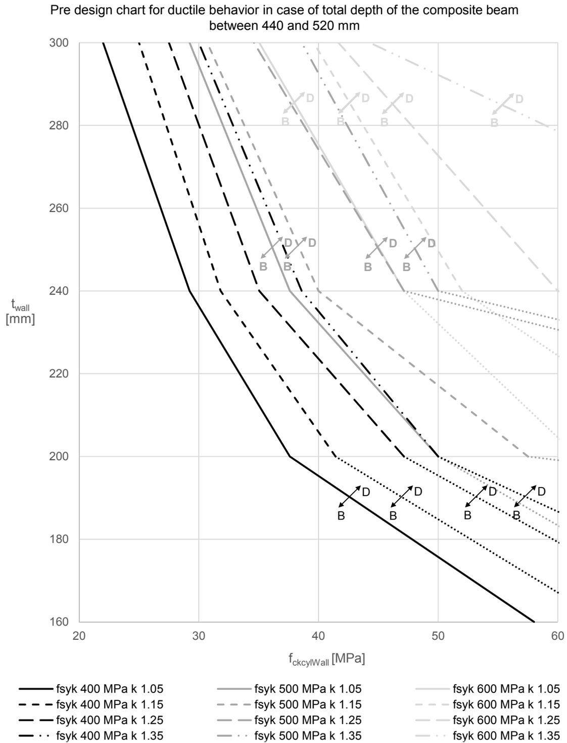
Fig. 4.60: Pre design chart for ductile behaviour in case of total depth of the composite beam between 440 and 520 mm
