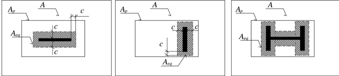
Fig. 3.8 Effective area under the base plate
