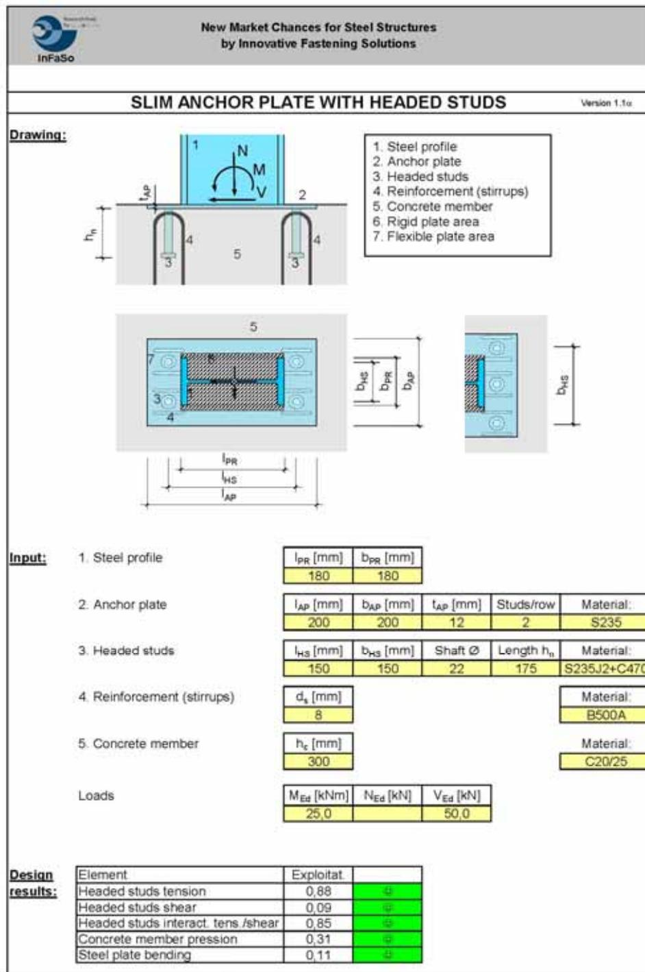
Fig. 3.12: Excel sheet, "Input+Output"-mask for version 1
