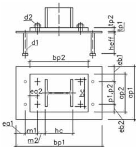
Fig. 4.43: Scheme of base plate with anchor plate
