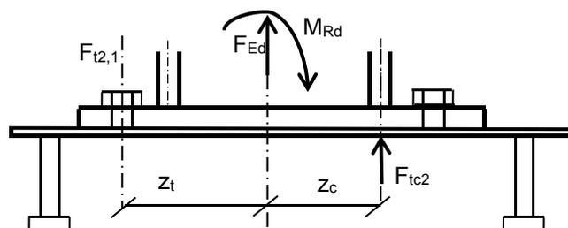
Fig. 9.23d The lever arm in tension and compression
