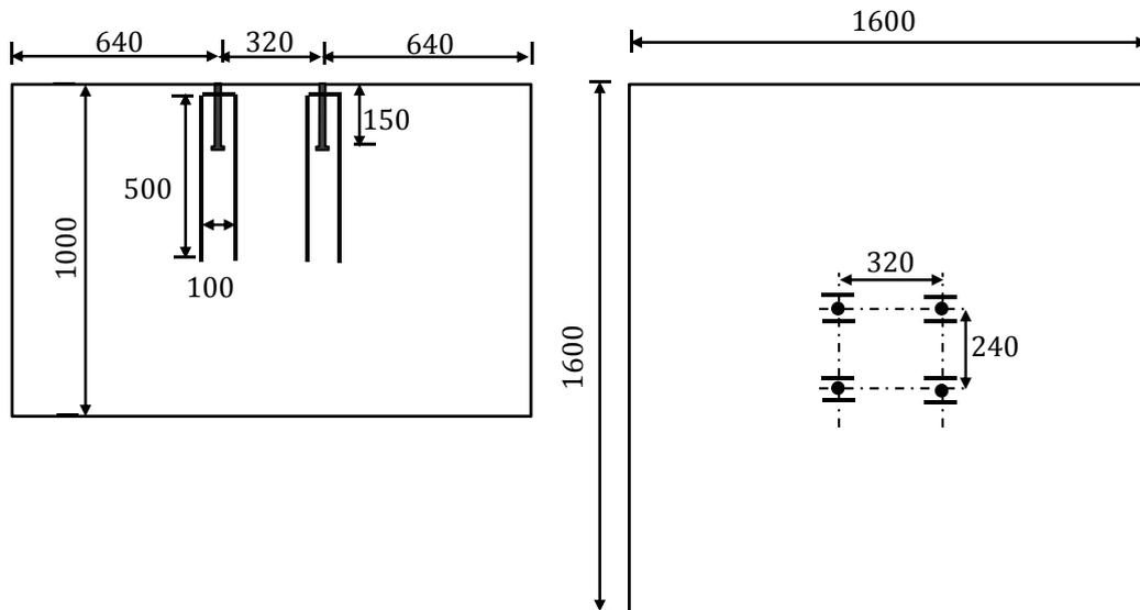
Fig. 9.6 Headed studs and supplementary reinforcement configuration
