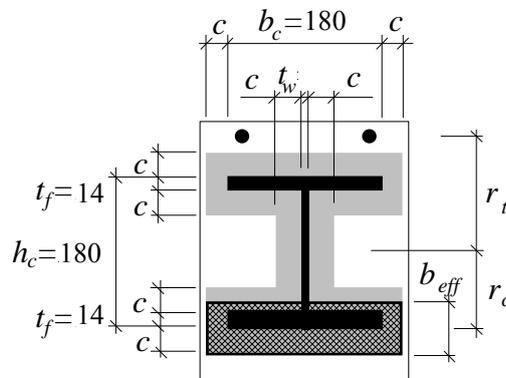
Fig. 9.42 The effective area under the base plate
