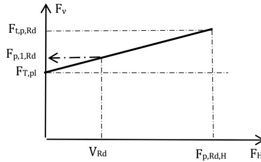
Fig. 4.19 Linear relation of vertical  $F_v$  and horizontal forces  $F_H$  at resistance
