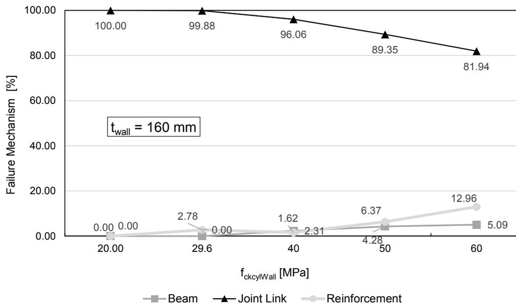
Fig. 4.55: Influence of wall concrete grade for  $t_{wall} = 160$  mm
