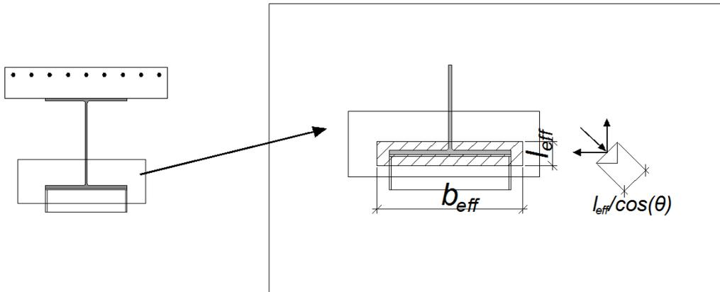
Fig. 9.31 Definition of the width of node N2
