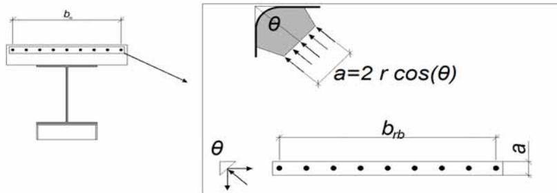
Fig. 9.30 Definition of the width of node N1
