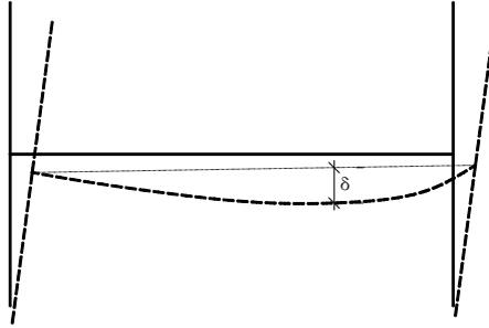
Fig. 7.9 Representation of the considered beams deflection
