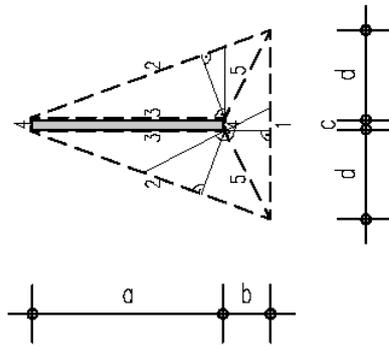
Fig. 2.14: Geometry for local rotating yielding lines
