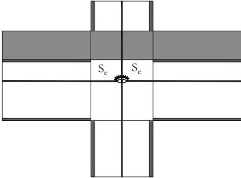
Fig. 7.1c Representation of joint by two rotational springs
