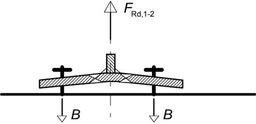
Fig. 4.7 T-stub without contact with the concrete foundation, Mode 1-2
