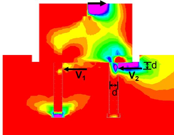
Fig. 5.6 Stress distribution  $\sigma_x$  in load direction
