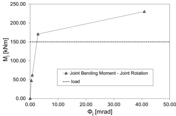
Fig. 9.33 Joint bending moment-rotation curve  $M_j - \Phi_j$
