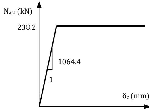
Fig. 9.7 Load-displacement behaviour of spring representing component S
