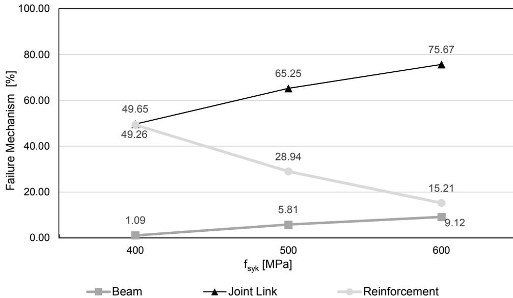
Fig. 4.47: Influence of yield strength of slab reinforcement
