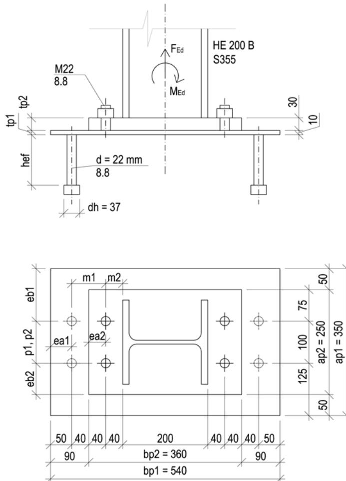
Fig. 9.19 Designed column base with anchor plate
