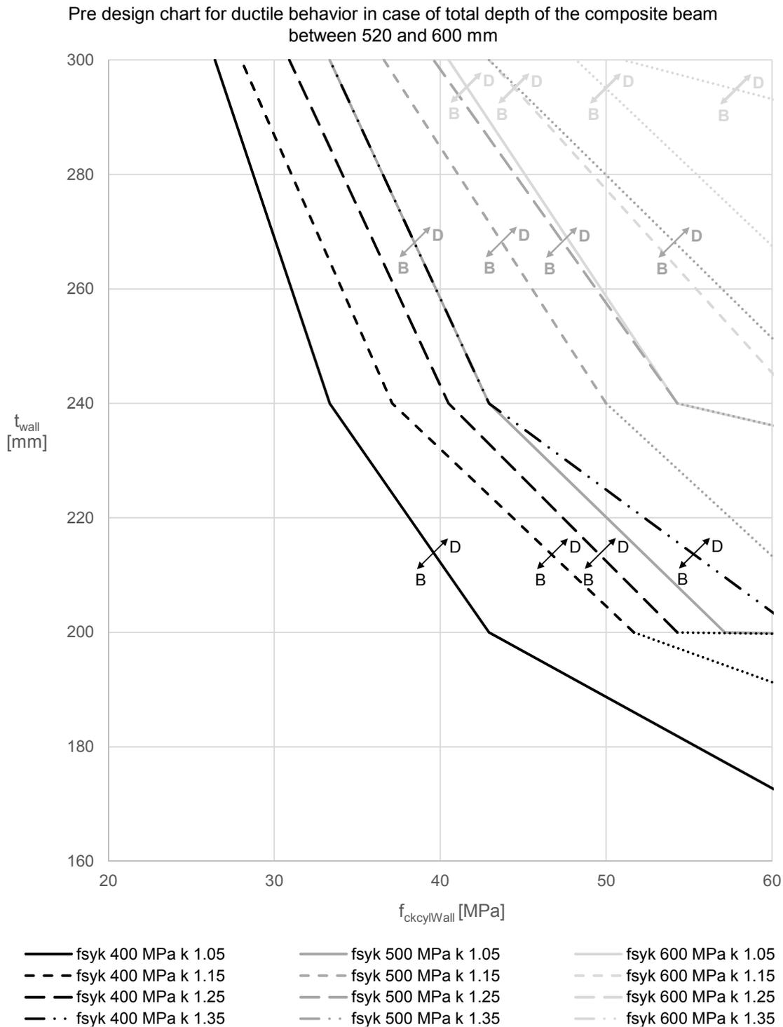
Fig. 4.61: Pre design chart for ductile behaviour in case of total depth of the composite beam between 520 and 600 mm
