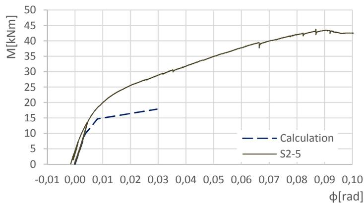
Fig. 4.29: Comparison of predicted and measured moment rotational relation for experiment S2-5, eccentricity 354 mm
