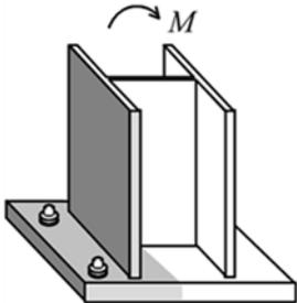
Fig. 4.3 Tensile zone and equivalent T-stub in case of loading by bending moment
