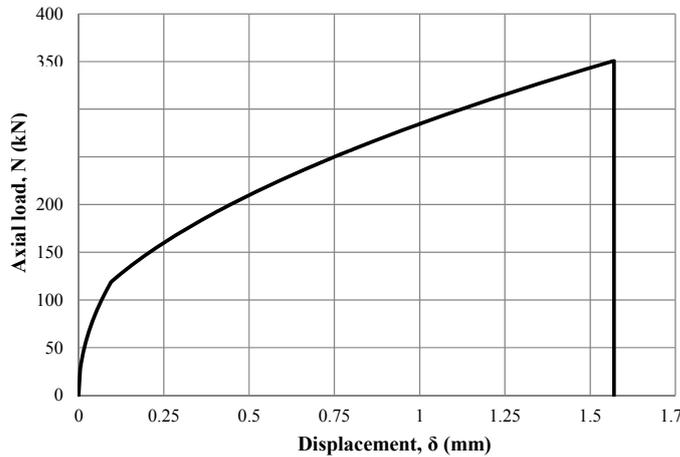
Fig. 9.12 Load-displacement behaviour of spring representing component P
