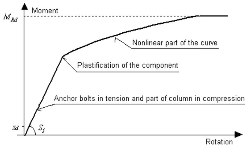
Fig. 6.4 Moment rotation curve for proportional loading
