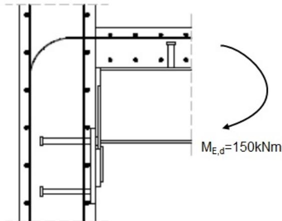
Fig. 9.27: Geometry of the moment resisting joint
