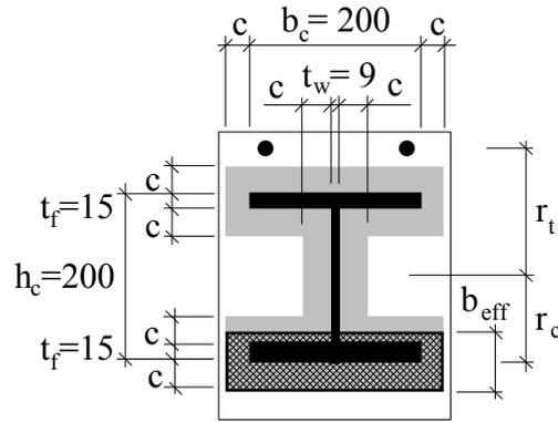
Fig. 9.4 The effective area under the base plate
