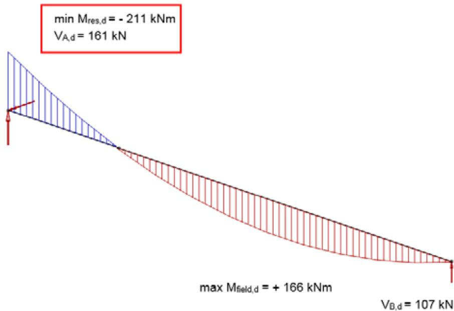
Fig. 3.8: Internal forces by taking into account the secant stiffness  $C_\varphi$  at the support A
