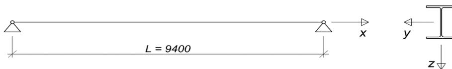
Fig. 9.25 structural system
