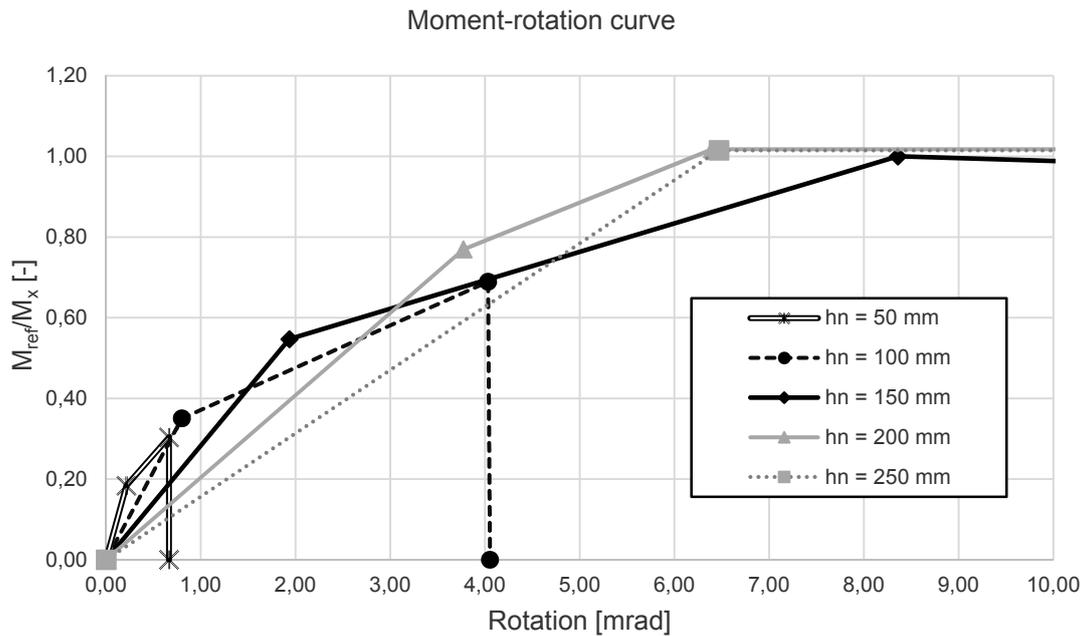
Fig. 4.15: Moment-rotation curve for variation of the effective height
