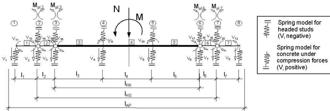
Fig. 2.9: Design model for vertical loads and bending moments
