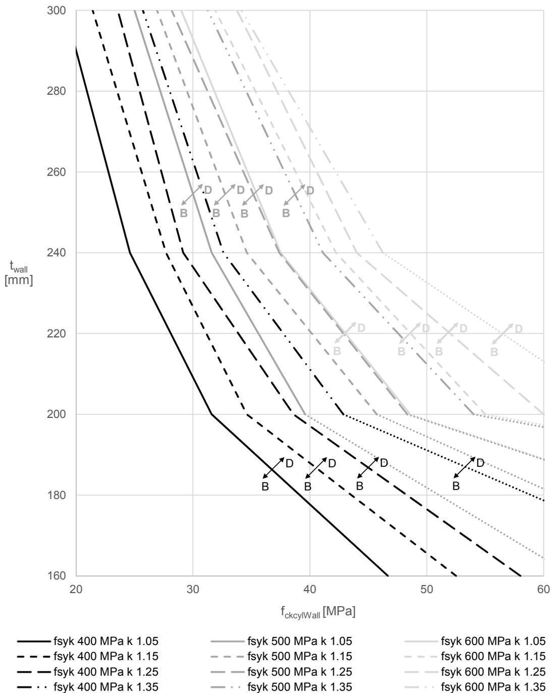
Fig. 4.59: Pre design chart for ductile behaviour in case of total depth of the composite beam between 360 and 440 mm
