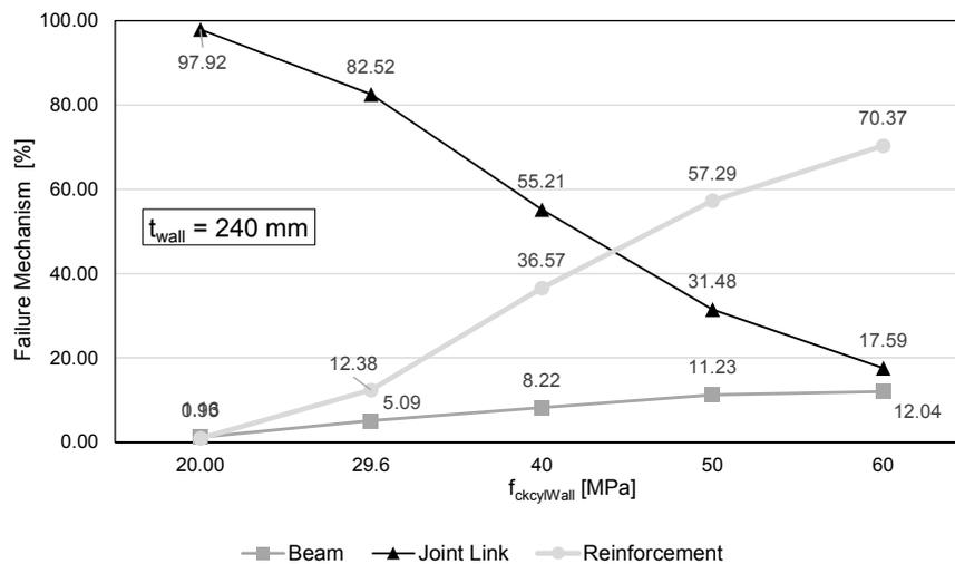
Fig. 4.57: Influence of wall concrete grade for  $t_{wall} = 240$  mm
