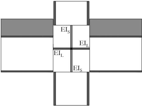
Fig. 7.1b Representation of joint by deformable stubs
