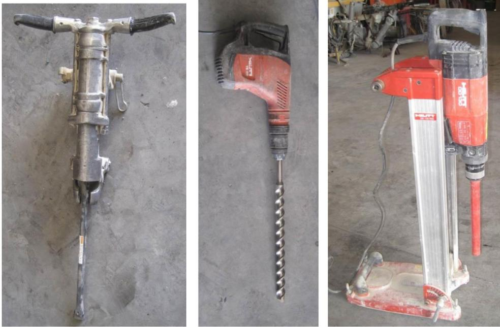
Fig. 3. The drilling machines used: pneumatic rock drill with compressed air, electrical hammer drill, and diamond core drilling.
