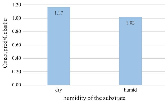
Fig. 10. Effect of the humidity conditions on  $C_{MAX}/C_{ELS}$  of horizontal anchors with epoxy and epoxy-acrylate fillings.
