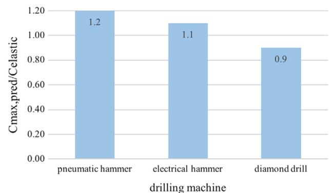
Fig. 7. Effect of the drilling machine on  $C_{MAX}/C_{ELS}$ .
