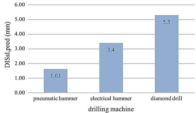
Fig. 14. Effect of drilling machine on displacement of the anchors.
