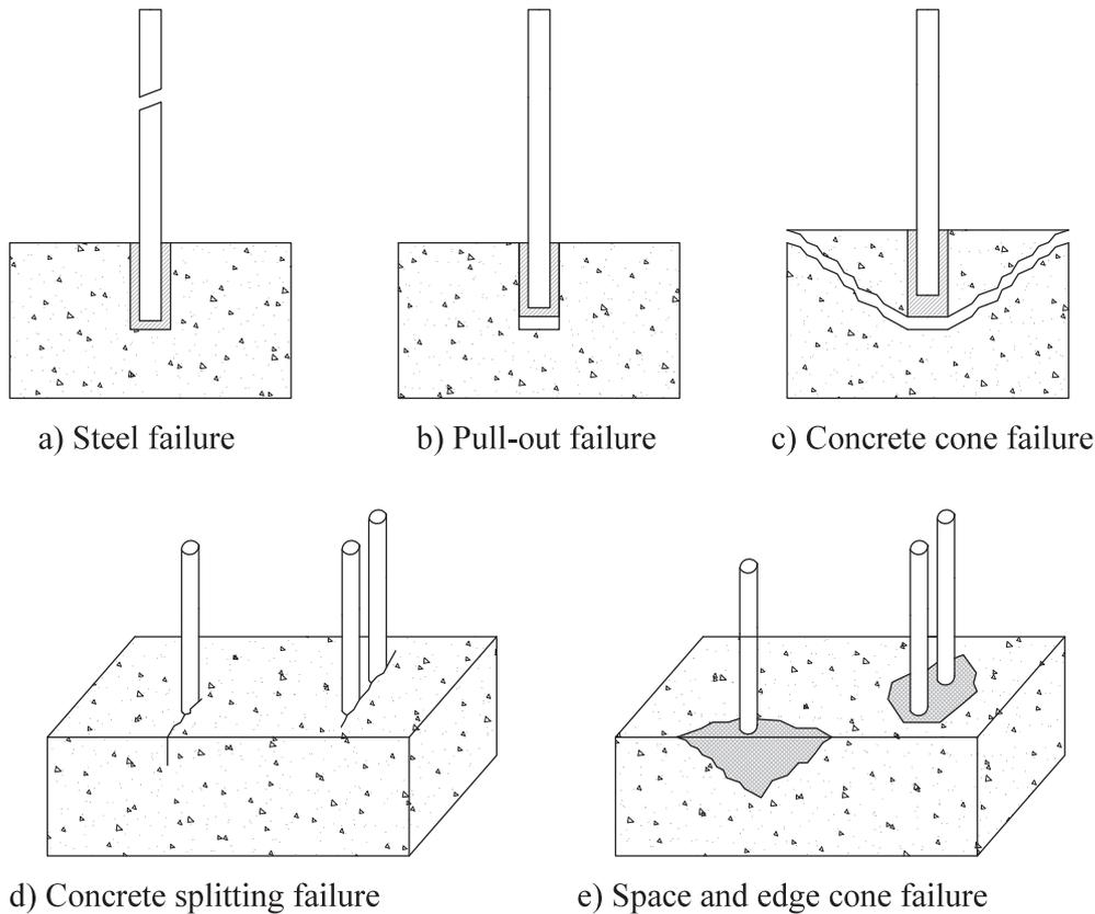
Fig. 1. Failure modes of adhesive anchors.
