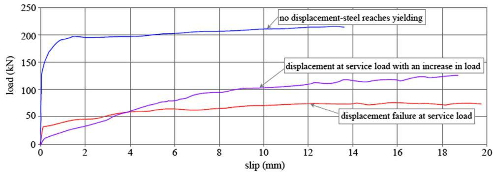
Fig. 5. Different load vs displacement curves. 1.
