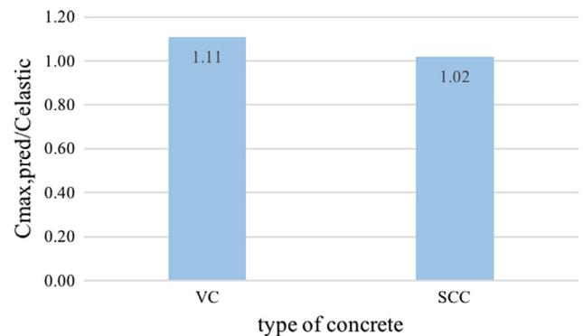
Fig. 6. Effect of type of concrete on  $C_{MAX}/C_{ELS}$ .
