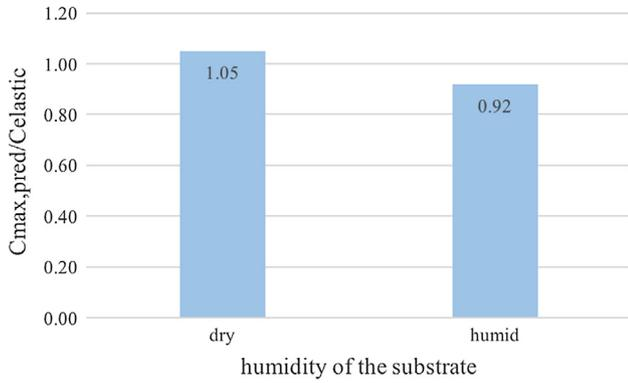
Fig. 12. Effect of the humidity conditions on  $C_{MAX}/C_{ELS}$  of anchors with grout.
