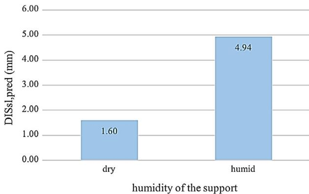
Fig. 18. Effect of moisture content on the displacement of anchors at service loads.
