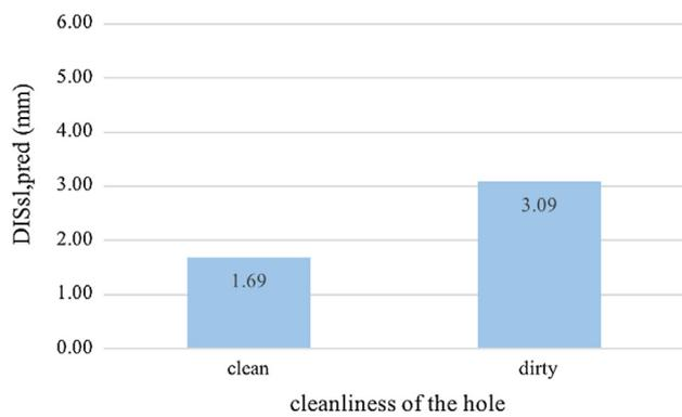
Fig. 17. Effect of cleanliness of the hole on the displacement of anchors at service loads.
