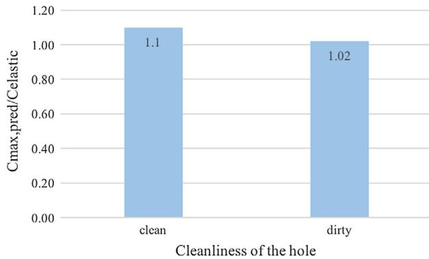
Fig. 9. Effect of cleanliness of the hole on  $C_{MAX}/C_{ELS}$ .
