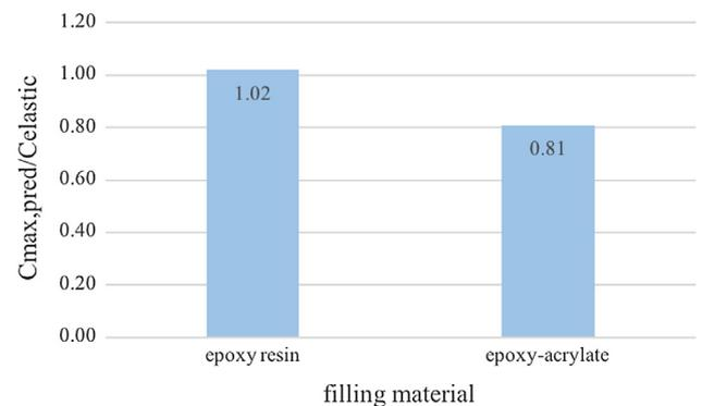
Fig. 8. Effect of filling material on  $C_{MAX}/C_{ELS}$ .
