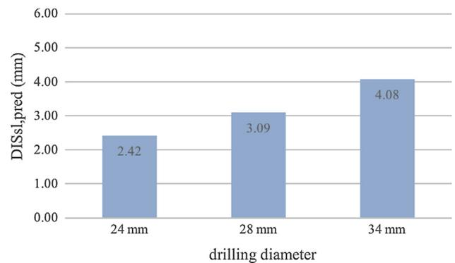
Fig. 15. Effect of drilling diameter on the displacement of anchors at service loads.
