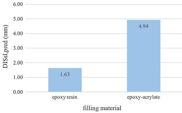
Fig. 16. Effect of filling material on the displacement of anchors at service loads.
