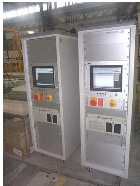
Picture No. 3: TEMA CONCEPT device, ALLTEST, intended for controlling the hydraulic jacks
