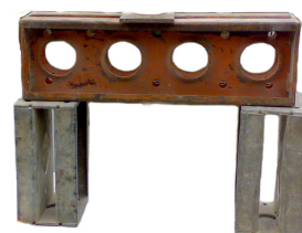
Figure 18 Heavy duty beam. Very heavy , but strong! For use with hollow ram and threaded rod.
