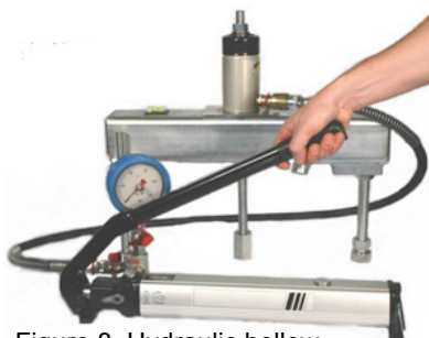
Figure 8. Hydraulic hollow cylinder mounted on heavy duty beam with adjustable legs with pump mounted gauge calibrated to 125kN. Load applied via threaded pulling rod connected to fixing by a threaded coupler. Can also use a pulling frame.
