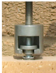
Figure 12 Bolt testing adaptor used with top hat adaptor to test anchor with projecting thread.
