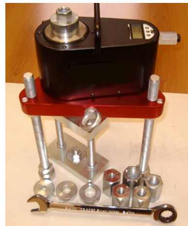
Figure 9 Hydraulic hollow cylinder with integral pump and digital readout calibrated to 145kN, mounted on a tripod with adjustable legs. Load applied via pulling frame. Threaded couplers also shown.
