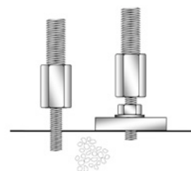
Figure 14 Threaded couplers. The arrangement on the right can demonstrate clamping force.
