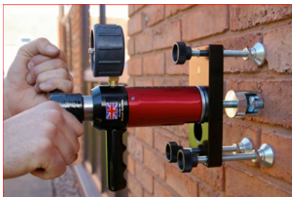
Figure 7. Light duty tester 0 – 30kN shown mounted to bridge which spans a complete brick course and thus also tests the mortar joints. Bolt type anchor being tested via special adaptor.
