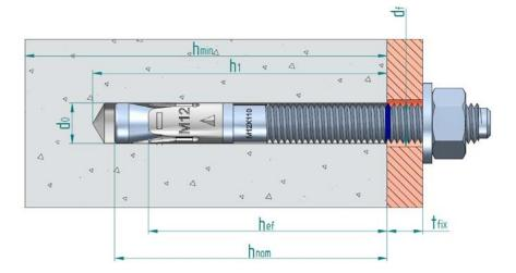
$\begin{array}{ll} d_0 \colon & \text{Nominal diameter of drill bit} \\ d_f \colon & \text{Fixture clearance hole diameter} \\ h_{\text{ef}} \colon & \text{Effective anchorage depth} \end{array}$
