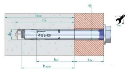
$\begin{array}{ll} d_0 \colon & \text{Nominal diameter of drill bit} \\ d_f \colon & \text{Fixture clearance hole diameter} \\ h_{\text{ef}} \colon & \text{Effective anchorage depth} \end{array}$
